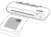
The finished sheet will emerge from the material exit ③ by itself. Remove it from the support rack only after it has completely cleared the exit.
